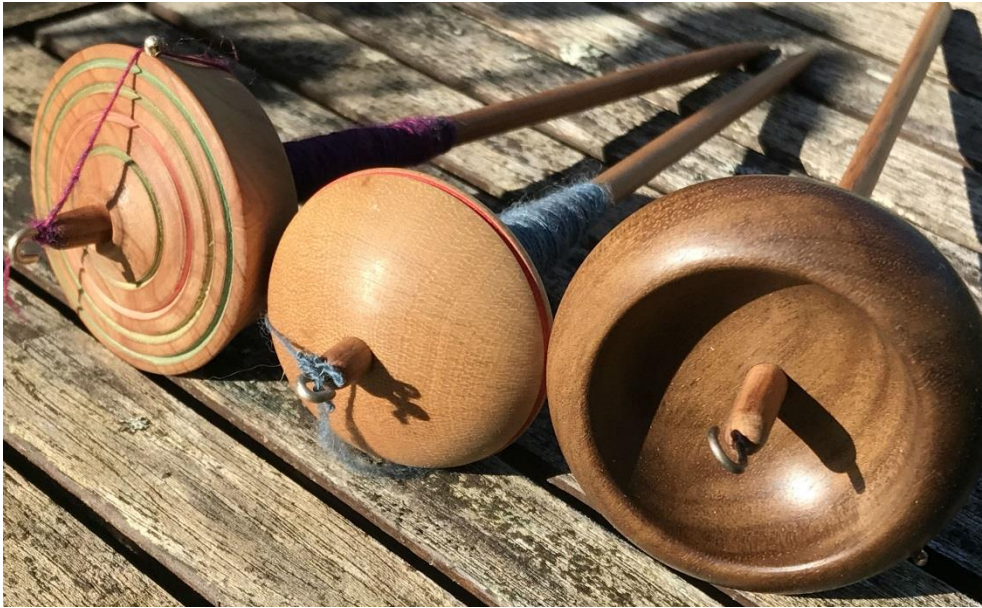
Figure 2 - a selection of high-whorl drop spindles made from New Zealand native woods.
