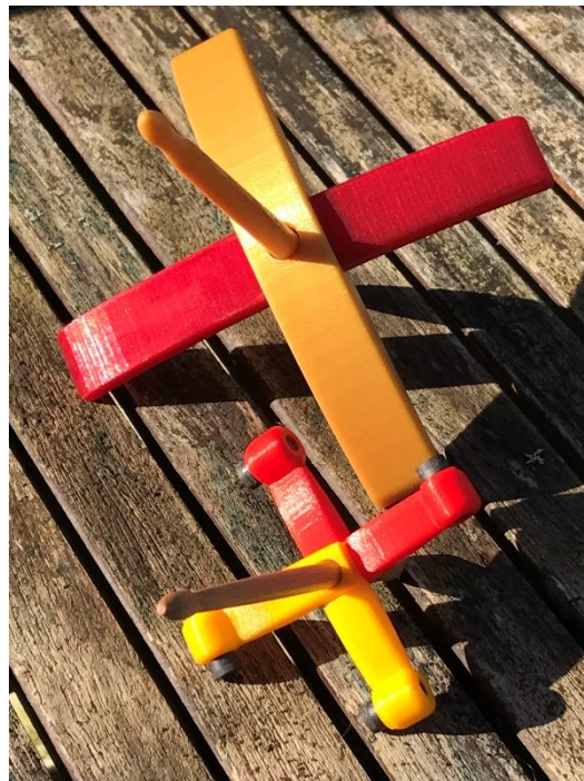
Figure 1- 3D printed Turkish spindles. Photo by the author.
