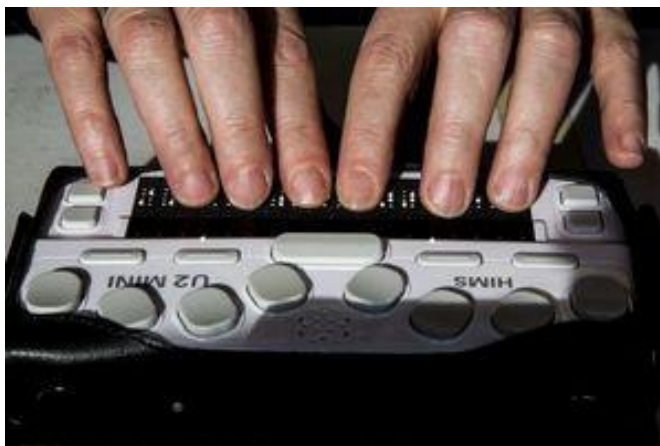
Sile O'Modhrain using electronic braille display Photo: (Joseph Xu) (Radio New Zealand 2016)
