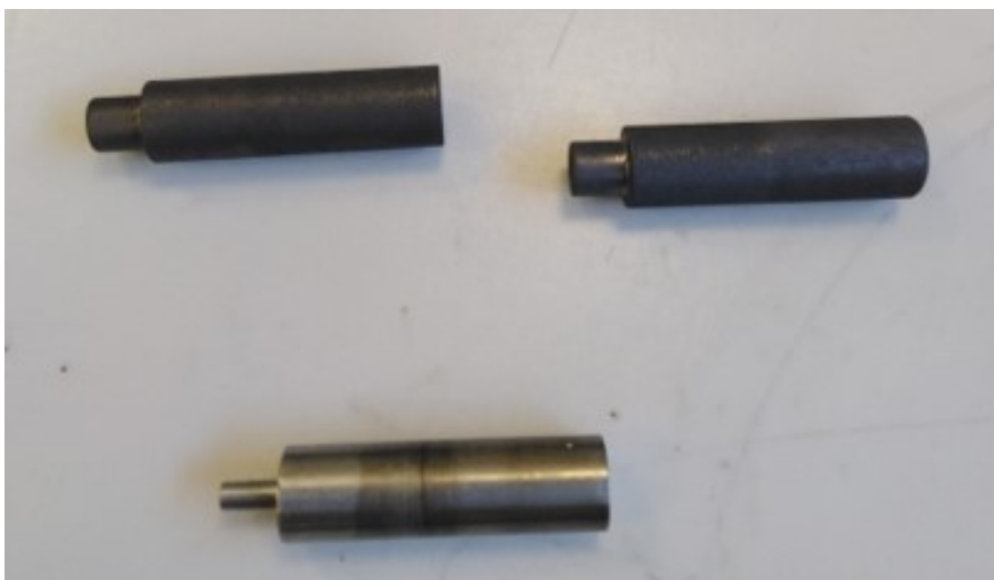
FIGURE 3.6: The graphite current collectors (top) compared to a Mo current collector (bottom). The graphite rods were manufactured to fit into the Swagelok-type cells that were available. 11 mm diameter and 5 cm long
