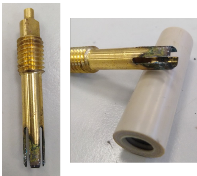
FIGURE 3.12: Corrosion on one of the brass connectors from a failed cell. This is assumed to be from a bad seal around the O-ring allowing electrolyte to leak into the chamber and react with the brass.
