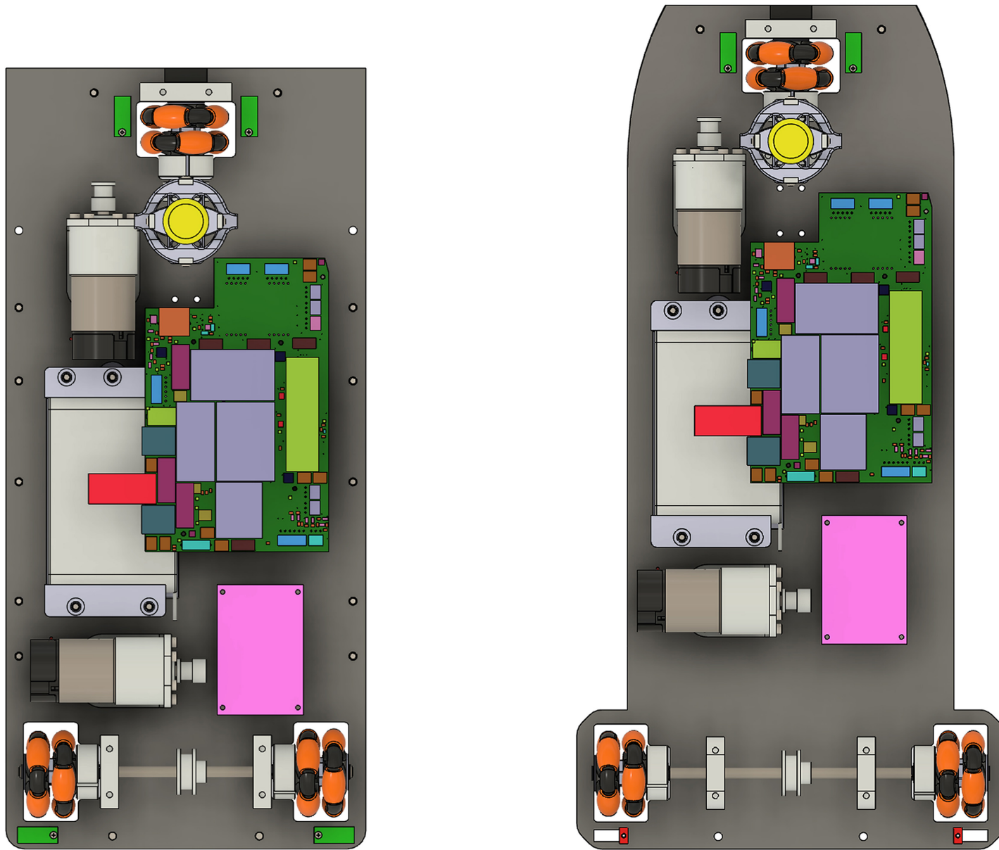
Figure 4.32. Baseplate and configuration of mechatronic components of the Mk.2 (left) and Mk.3 (right).
